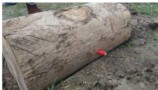
Plate2: Wooden Plank as the Vibration Source
