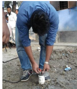
Plate5: Geophone Lowering In the Borehole
