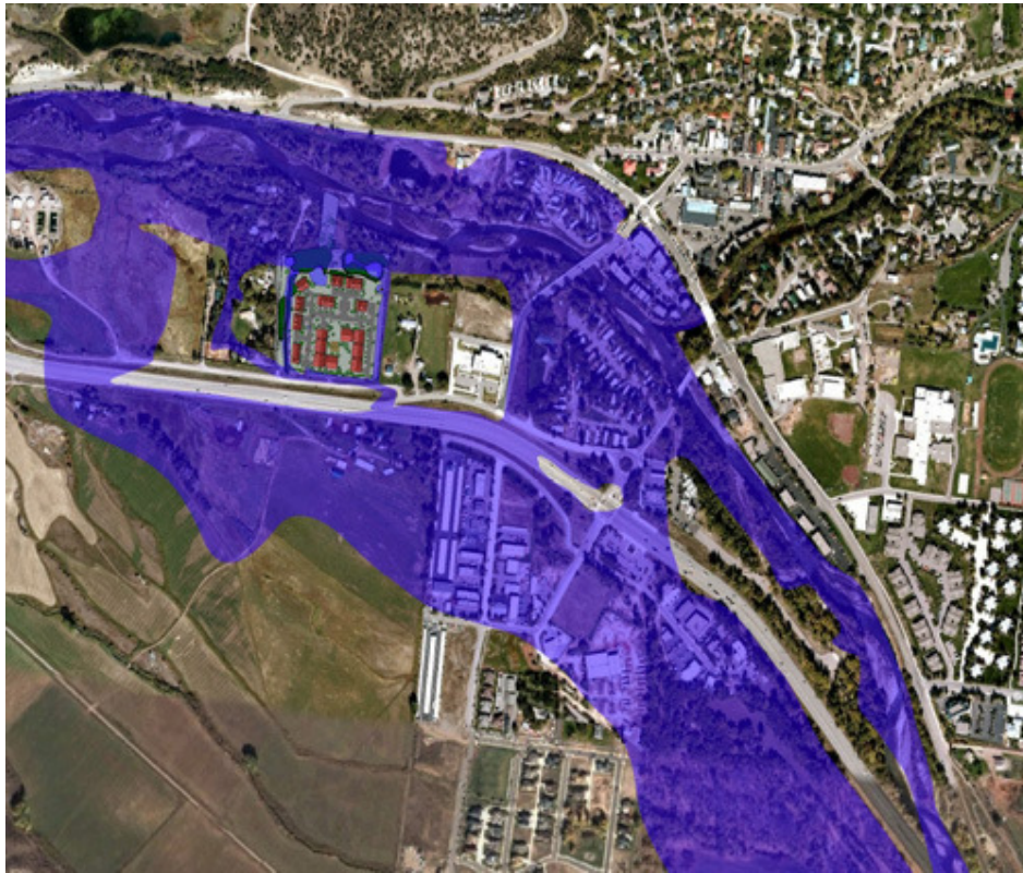
Figure 2-26: Water Surface TIN extracted During Floodplain Modeling
