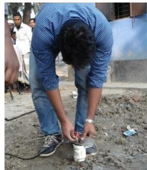
Plate5: Geophone Lowering In the Borehole
