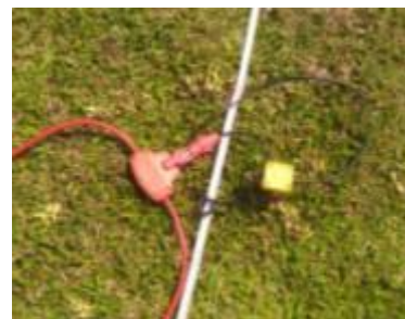
Vertical Geophone of 10 Hz capacity
