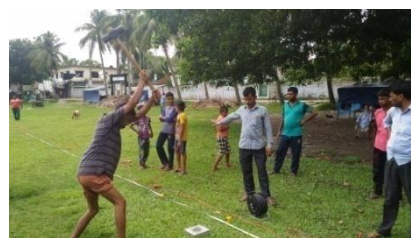
shoot it vertically by 8kg hammer to generated elastic waves
