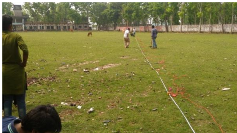
Set receivers along the line at the ground surface and the intervals of each geophone are 3m
