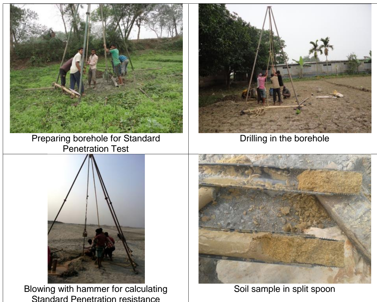
Plate 8: Standard Penetration Test Activity at Rangunia Area.
