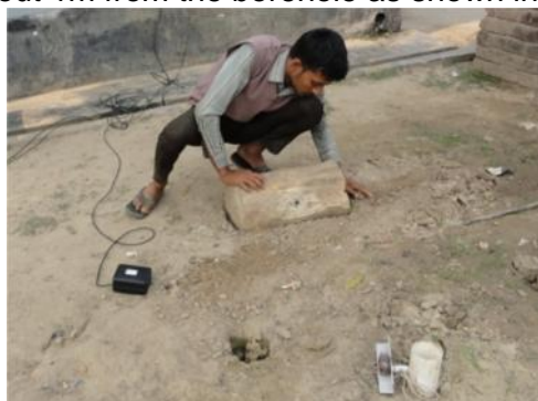
Plate2: Wooden Plank as the Vibration Source
