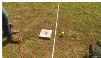
Vertical Geophone of 10 Hz capacity
